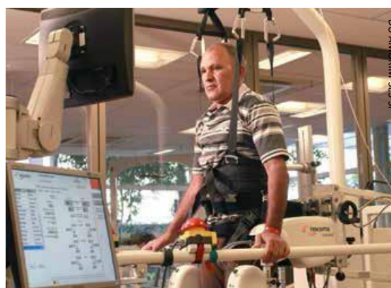
Use of the Lokomat, consisting in a brace that sustains the patients waist and two orthoses for the lower limbs.
