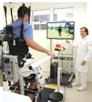
Lokomat, piece of equipment for rehabilitation of lower limbs - IMREA Vila Mariana
